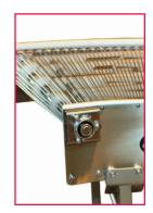
All bolt together connections have standoffs to aid in cleaning and minimize harbor points.
